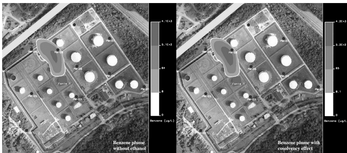
Figure 1 – Comparison of simulated plumes of benzene in groundwater due to a gasoline and ethanol spill scenario, considering the cosolvent effect and without presence of ethanol
