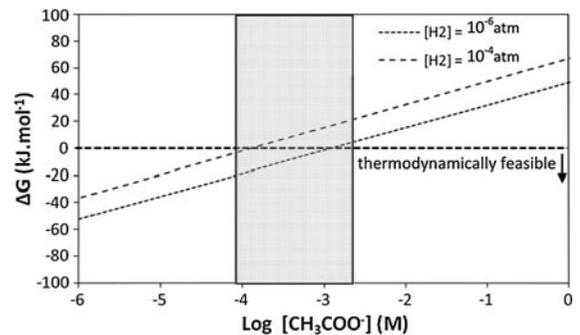
**Fig. 3** Thermodynamic feasibility of benzene fermentation ( $0.9 \text{ mg L}^{-1}$ ) to acetate and hydrogen (reaction 2) for a range of likely  $\text{H}_2$  concentrations ( $10^{-4}$ – $10^{-6}$  atm). Shaded area indicates the range of acetate concentration (max:  $\log -2.7$  M and min:  $\log -4.1$  M) measured in the biostimulated source zone
