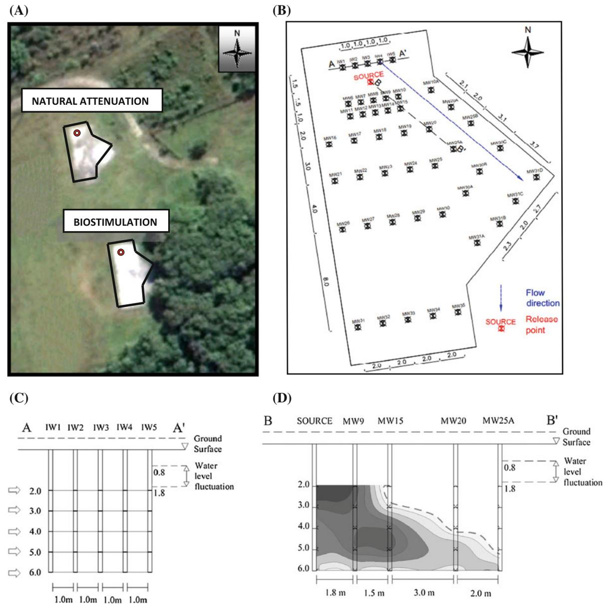
**Fig. 1** Plan view depicting the location of natural attenuation and biostimulation field experiments (a), schematic view of experimental areas configuration (b), cross sections of transect A–A' (c) and B–B' (d) from biostimulation plot. Arrows in transect A–A' (c) indicate the sampling depths where ammonium
